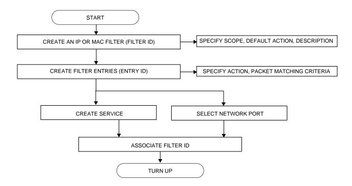
Figure 21: Filter Creation and Implementation Flow
